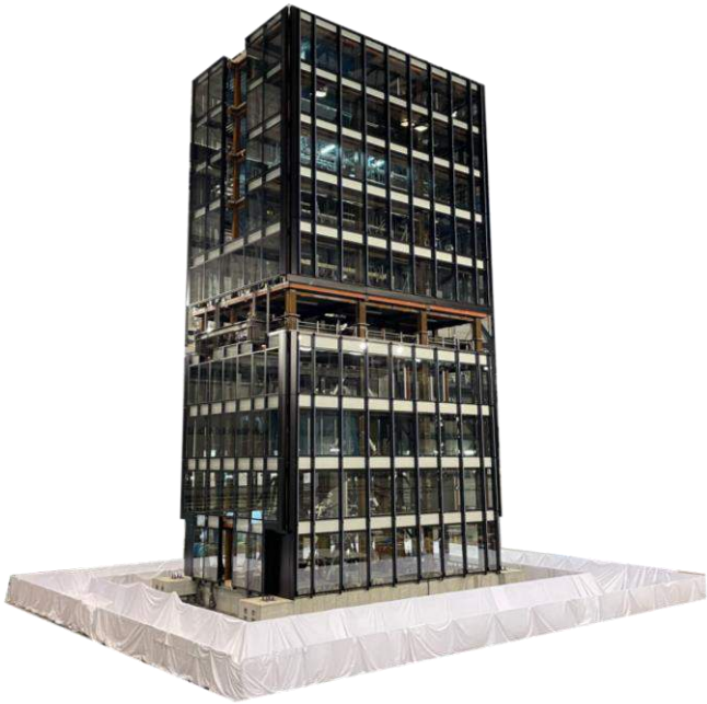
Study building (10-storey, full scale test)
