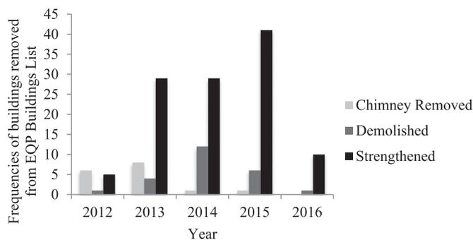
Fig. 1. Annual frequencies of commercial/public buildings removed from the EQP Buildings List, from years 2012–2016, due to chimney removal, demolition, or strengthening. Data for 2012 and 2016 are for six months only.
